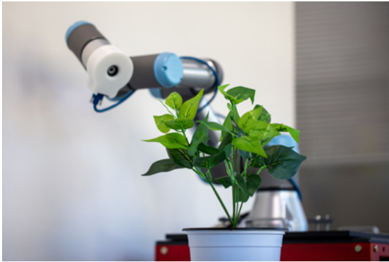
Robot system scanning 2D plant images
