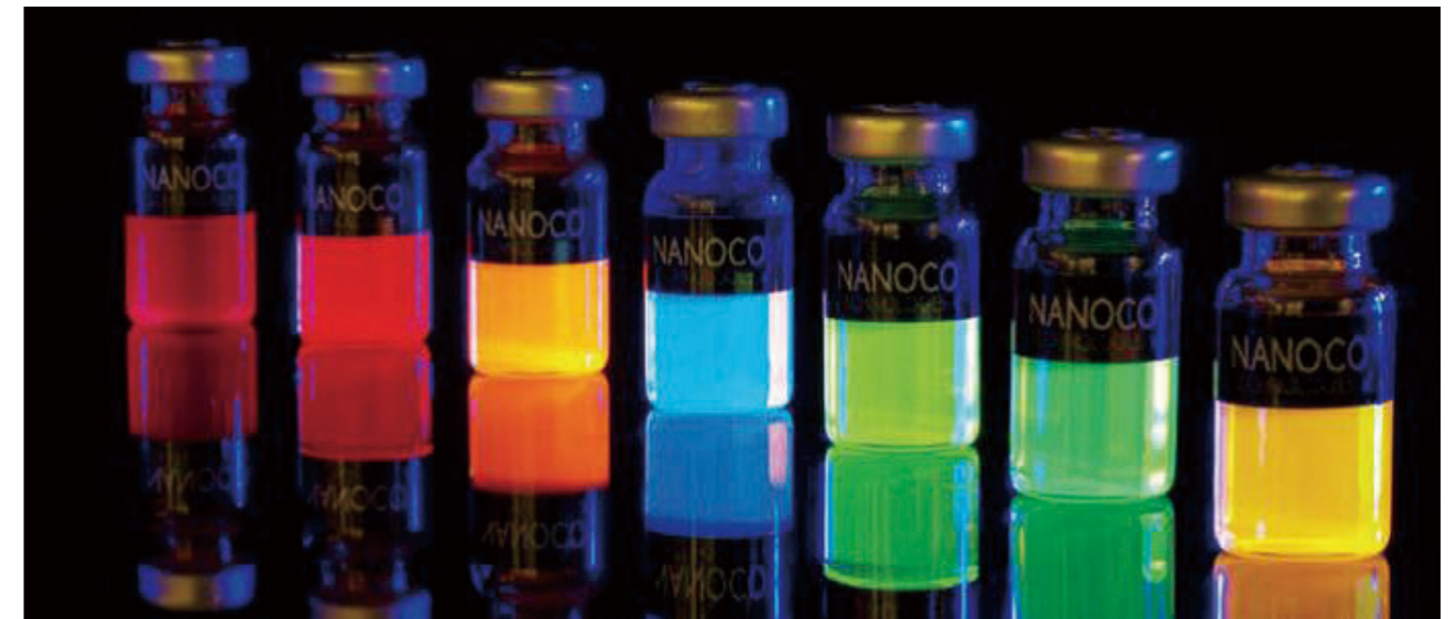
Figure 1. Colloidal quantum dots (CdSe/ZnS core shell type).
