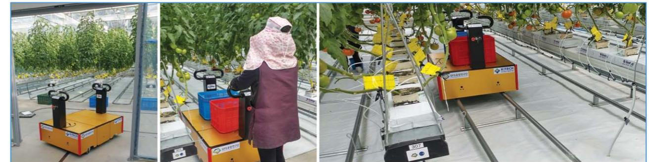
Figure 4 Transport robot for greenhouses.
