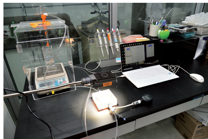
The membrane is on testing for biofouling removal under an LED lamp
