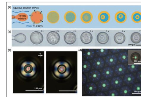
Multiple emulsion drops containing cholesteric liquid crystal through phase separation process and their reflection colors
