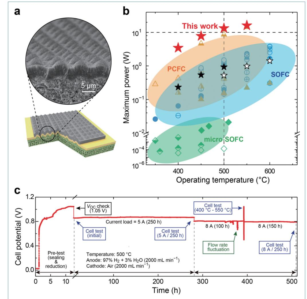
(a) Cross-sectional SEM and schematic images of a 3D SOFC cell. (b) Comparison of the total power performance in this work with that of the previously reported ceramic fuel cells. (c) Long-term stability test results of a large-area 3D SOFC at 500°C.
