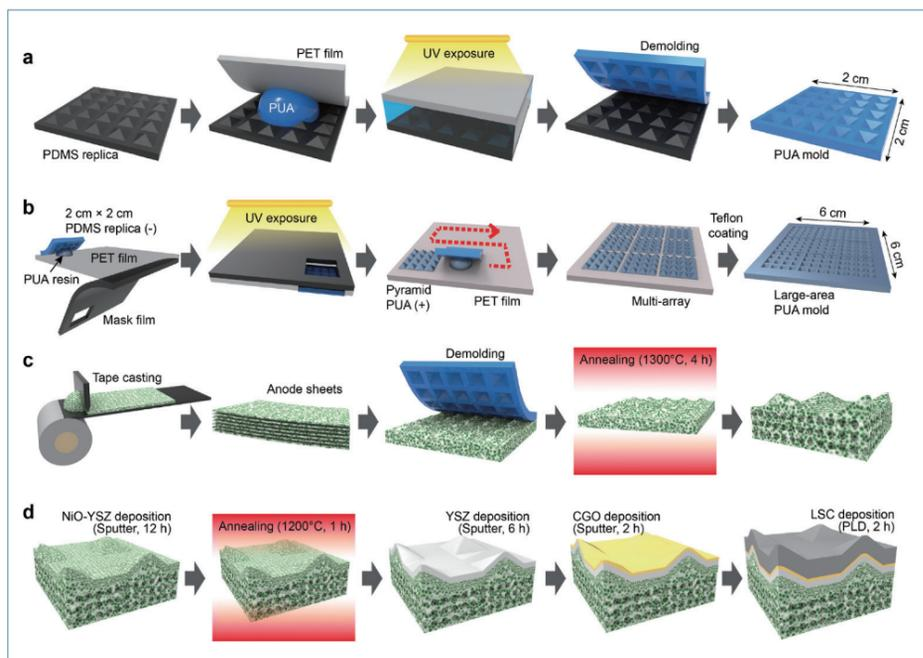
Schematic illustrations regarding the (a) preparation of a small PUA mold from a PDMS replica, (b) preparation of large-area PUA mold (c) molding process to fabricate a 3D patterned substrate, and (d) deposition of several thin-film layers.
