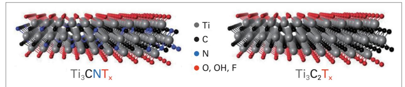
Schematic representation of the  $Ti_3CNT_x$  and  $Ti_3C_2T_x$  MXenes.  $T_x$  represents surface terminations (-OH, -O, and -F)
