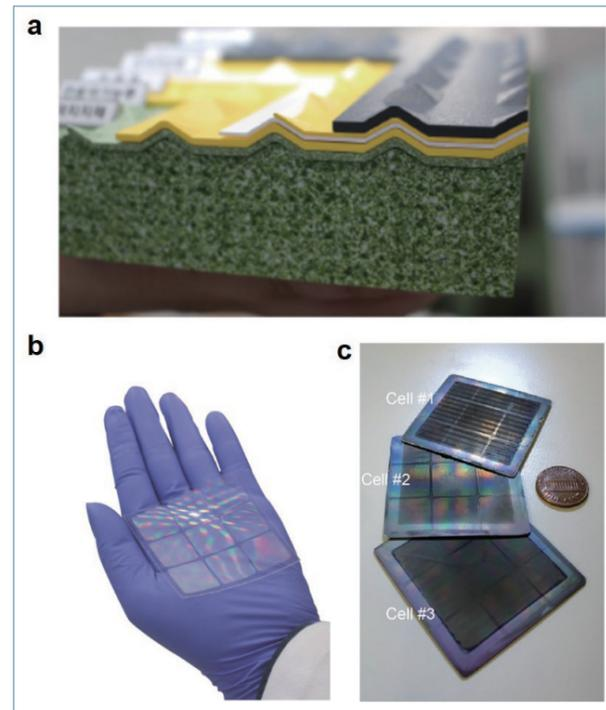
Images of the (a) cutaway model showing 3D interface structures, (b) large-scale PUA mold, and (c) three large-area 3D SOFCs after electrochemical performance tests.
