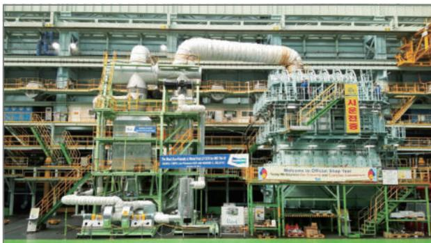
**Figure 2.** The world 1<sup>st</sup> official shop test of the LP SCR catalyst system was carried out with a marine engine of Doosan Engine co.
