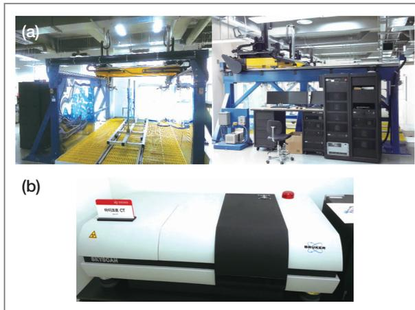
**Figure 8.** (a) 3D C-Scan and (b) Micro CT equipment at KIST Jeonbuk.
